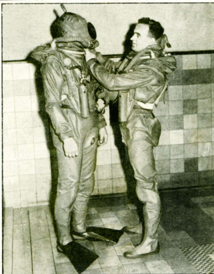
BRITISH "FROG-MAN" READY TO GO UNDER has his "fish" suit adjusted by a Petty Officer (right). Existence of these underwater Commandos, known as L.C.O.C.U. (Landing Craft Obstruction Clearance Units), was only recently disclosed. Special breathing apparatus enables them to remain under water for 1 1/2 hours at a stretch, their "fins" giving them a speed of 60 yards a minute. On D-Day, they removed from the Normandy beaches mines and other obstructions. See also page 341. Photo, Special Services.
