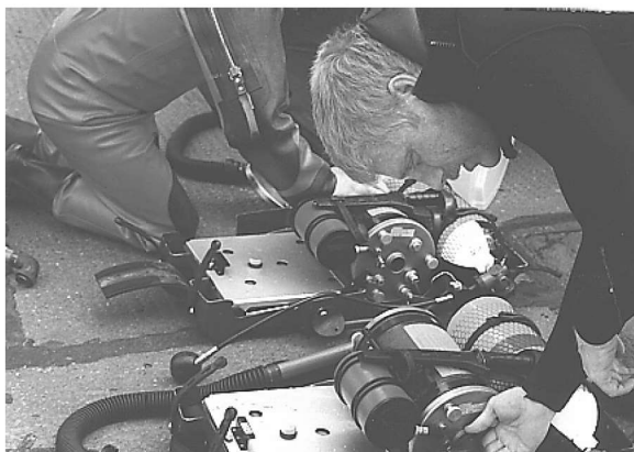
AGAs ACSC (Alternativ Closed, Semi-Closed) klar-gøres
